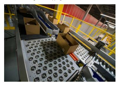
Orders are routed via conveyor to the packaging area where invoices are inserted, lids are put onto boxes automatically, shipping labels are applied, and all orders route to a shipping sorter for sortation to the final destination.
