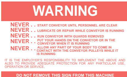
PLACED AT DRIVE OF ALL POWERED CONVEYORS.
